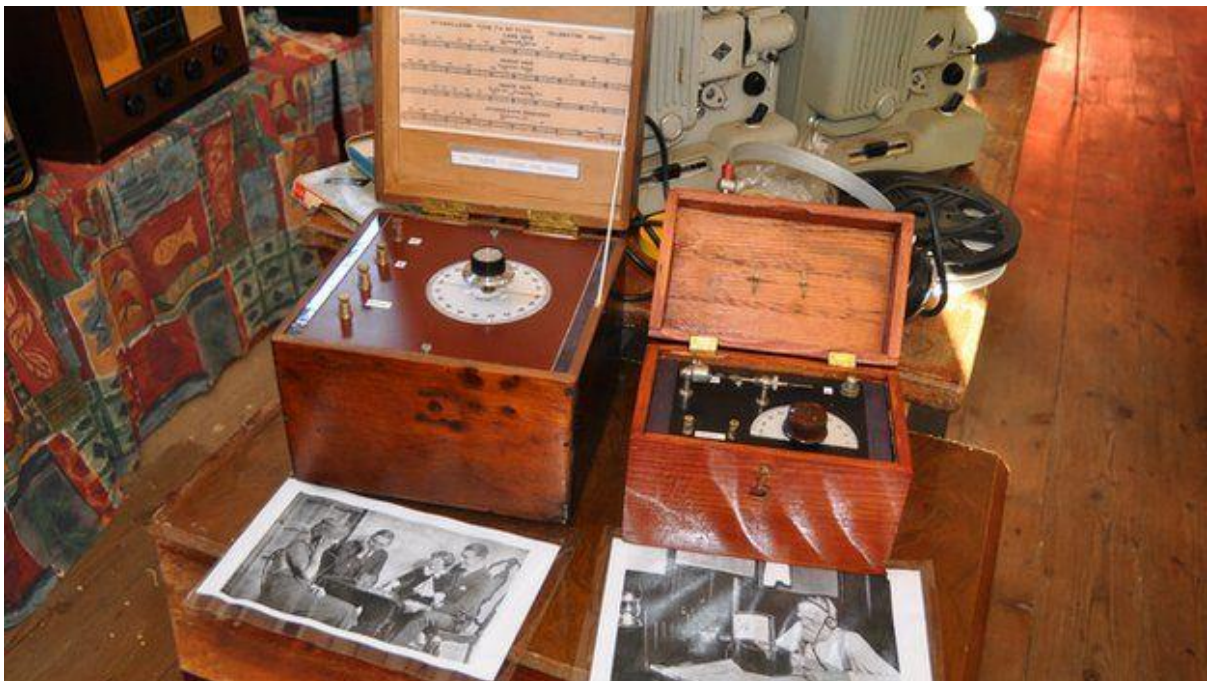
Crystal sets from about 1900 only had headphones rather than loudspeakers
